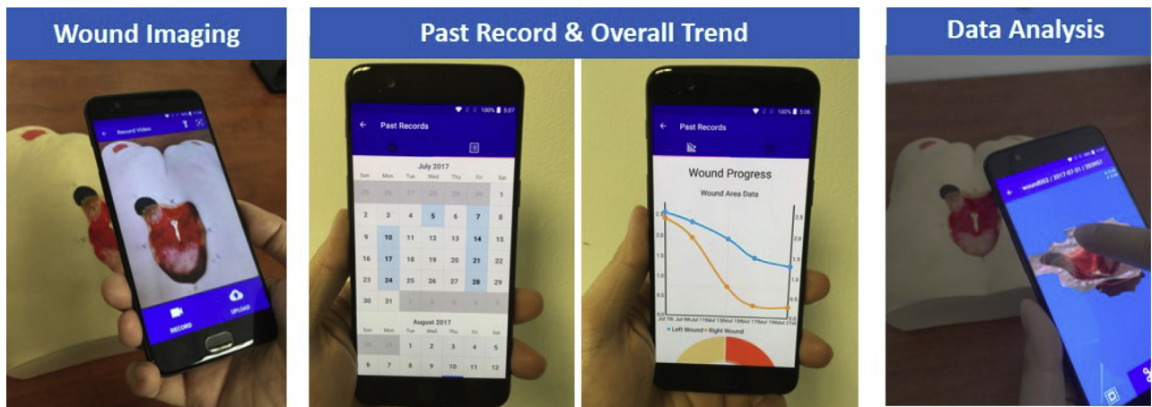
Figure 5 Preliminary iDr app for wound imaging, wound record, trending, and 3D analysis.
