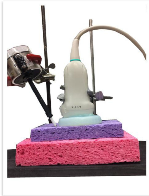
Fig. 1. Experiment setup photo. An ultrasound probe was put atop an ultrasound gel pad to measure the surface wave speed of the lung phantom—the purple sponge. The pink sponge and the black rubber were put under the purple sponge to reduce the reflection of the sound wave from harder surfaces. A shaker was in contact with the purple sponge surface to generate harmonic vibrations on the sponge surface. The bars behind the shaker and the ultrasound probe are the holder frames used to keep the equipment in place.
