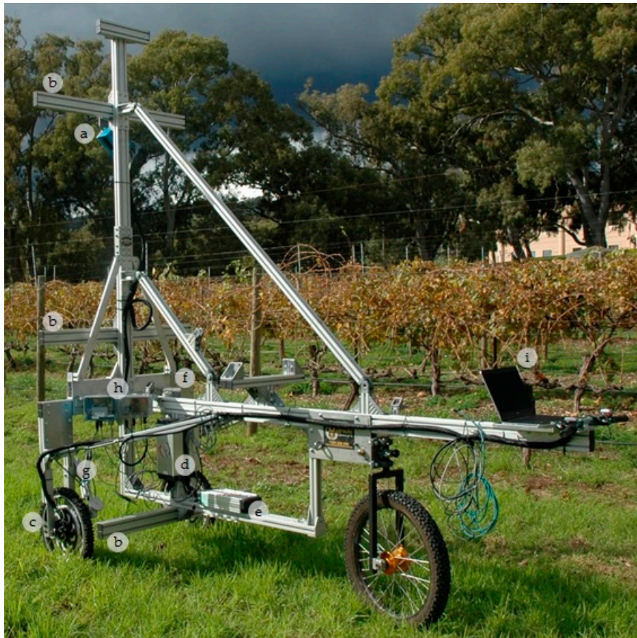
Figure 1. This shows GRouter's frame and components: (a) is the SICK LMS-400 light radar (light detection and ranging, LiDAR), mounted 2.25 m above the ground at a 45-degree angle. The LiDAR scans at 250 Hz at a wavelength of 650 nm and a range of 3 m; (b) shows the masts on which instruments can be mounted—each mast can be moved up, down, away from or toward the frame; (c) each of the front wheels contained an electric motor; (d) shows the 48v batteries used to power the wheels; (e) is the 24v instrument battery which was split into separate voltages by (f) the junction box; (g) is the spring-armed wheel encoder, which tracked the linear distance travelled during scans; (h) the data from the LiDAR, encoder and Global Positioning System with Inertial Measurement Unit (GPS/IMU), which was attached to the top of the LiDAR, were relayed back to (i) the field laptop.
