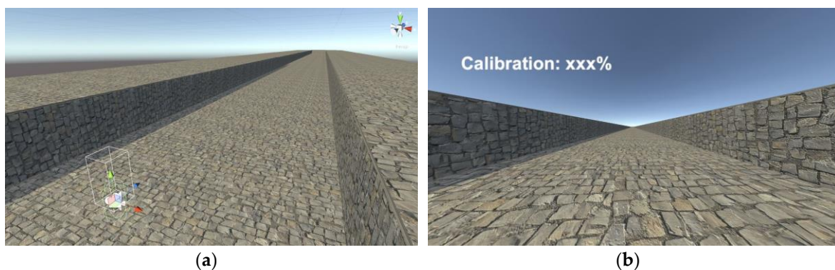
Figure 13. A 20 \times 400 \text{ m}^2 virtual space surrounded by walls: (a) a map with a bird's-eye view, and (b) a scene and a user interface (UI) viewed through the display of the HMD.
