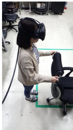
Figure 15. When performing WIP, a user could grab or lean on something to maintain balance. A subject preparing to complete a task. Using a chair with handles, the subject maintains balance. The chair is fixed so it cannot be pushed.
