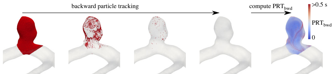
Figure 2. Tracers are seeded on the computational nodes in the region of interest (aneurysmal region). The tracers are integrated backward in time until they leave the region of interest. Subsequently, backward RT is calculated and mapped to tracer initial location. The red dots demonstrate tracers that are initially densely seeded in the aneurysm and subsequently integrated backward in time.
