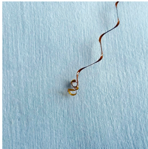
Figure 8. Delamination of the coverlay and curling of the FCB materials after tensile tests performed on the interconnects.
