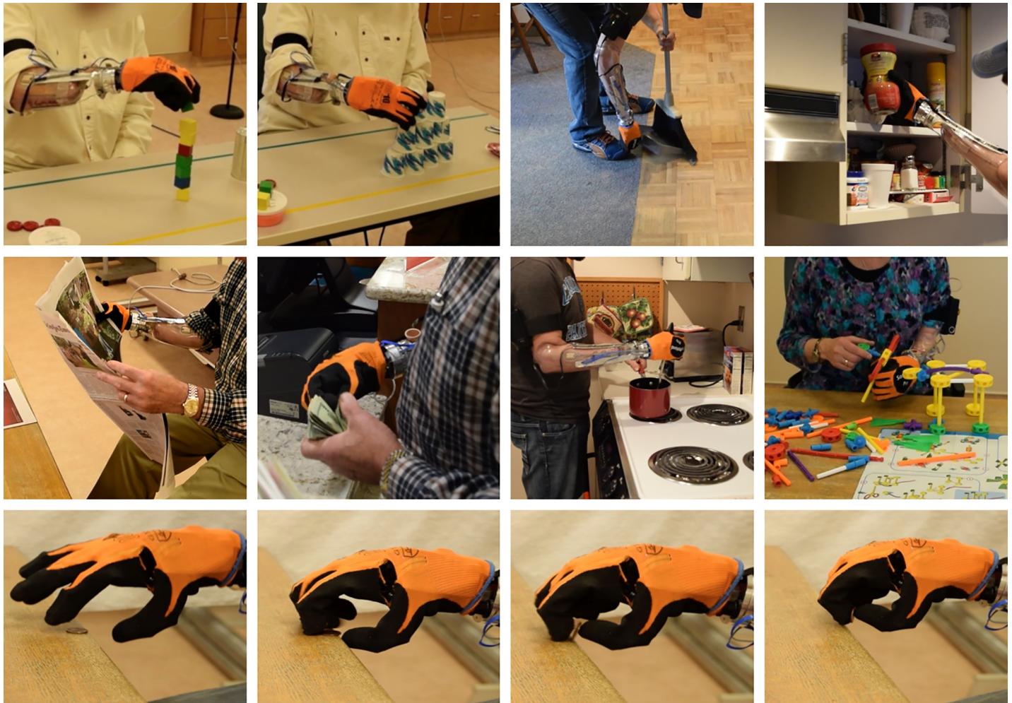
Fig 4. SoftHand Pro training. An example progression through training starting from simple, repeated grasp tasks (top row, left two) to real-world tasks exploring the work space (top row, right two) to coordinated bimanual tasks, including hobby and leisure activities (middle row). The bottom row shows a participant practicing using environmental constraints to pick up a coin (US penny) from a table. The movement (left to right) starts with pre-grasping, proceeds to blocking the thumb against the table edge, closing the fingers to meet the table and coin, sliding the coin to the edge while bringing the thumb up to meet it, and ends with grasp completion.
