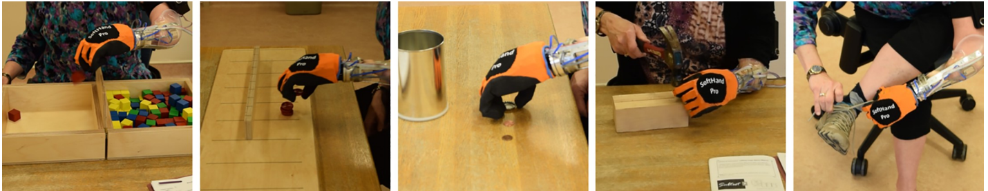
Fig 3. Clinical evaluation of prosthesis. Examples of participants completing the clinical measures. From left to right, Box and Blocks, the Jebsen Taylor Test of Hand Function (stacking checkers, moving small, common objects), and the AM-ULA (hammering a nail, shoe tying).
