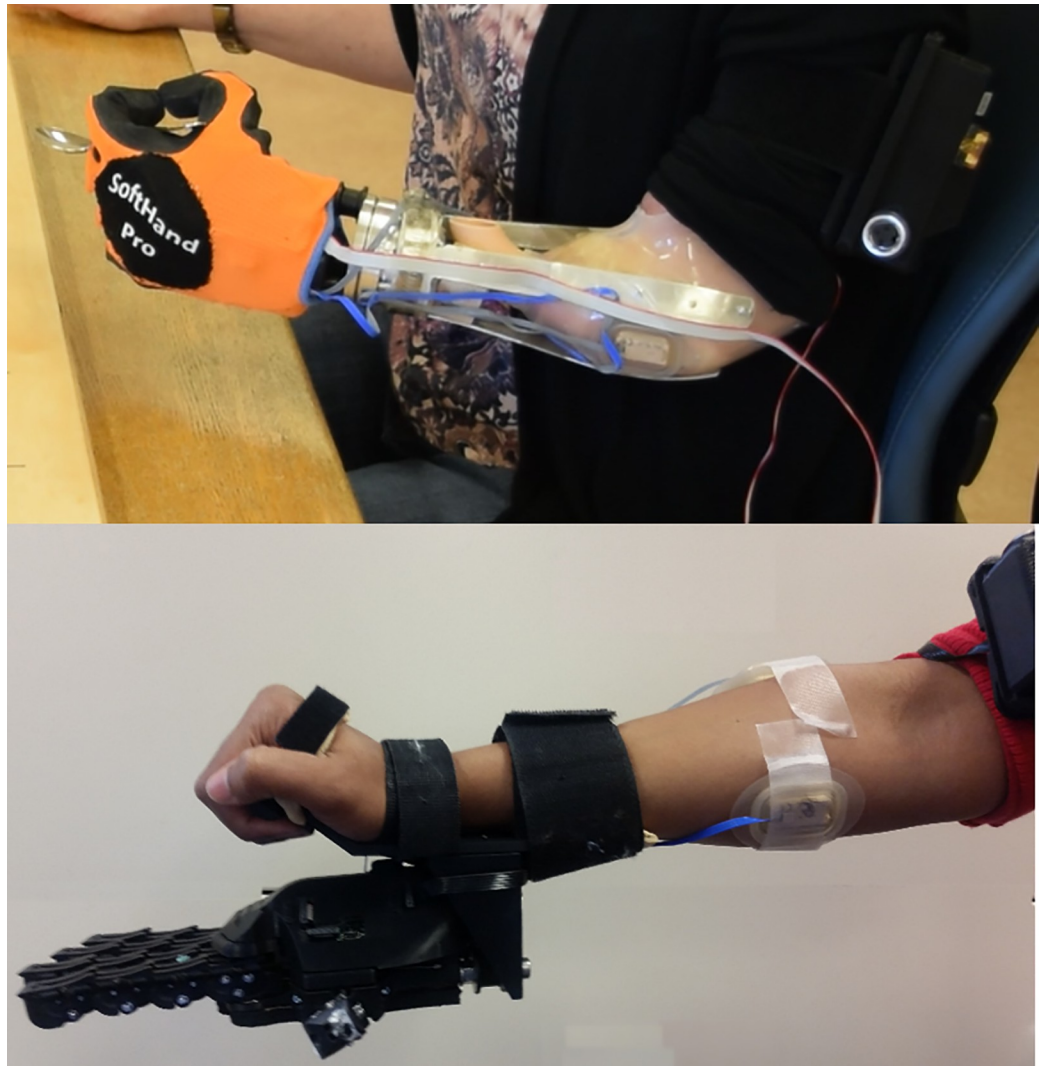
Fig 2. Participants wearing the SoftHand Pro. Top: The SHP attached to a myoelectric socket used by a participant with limb loss. Bottom: The SHP attached to a forearm adapter used by limb-intact participants.
