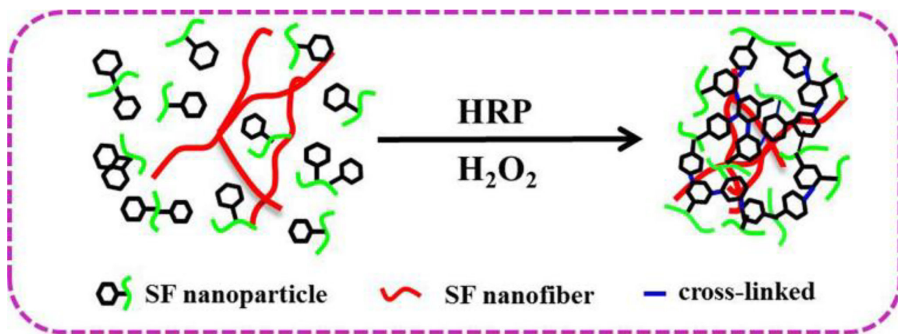
Figure 1. The mechanisms and structure of silk fibroin nanofiber-reinforced hydrogels prepared via the enzymatically crosslinked process. HRP is horseradish peroxidase for the crosslinking reaction.
