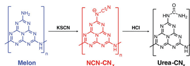
Figure 4. Reaction scheme of inserting oxygen-functional group in carbon nitride. Reproduced with permission. [44] Copyright 2017, Wiley-VCH.
