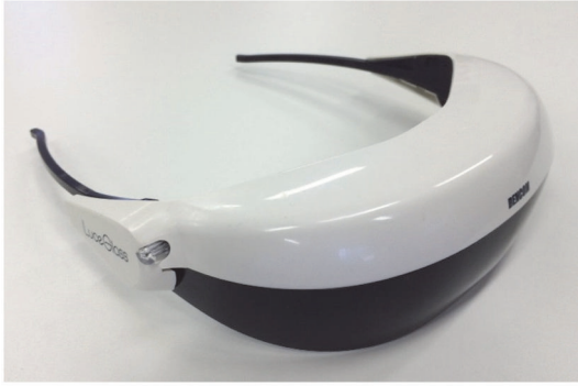
FIGURE 1: Goggles for bright light therapy. LEDs at the back of the frame are used as the light source.
