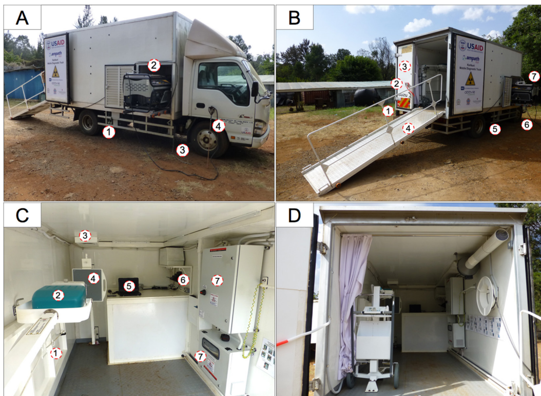
Figure 2 Mobile diagnostic unit equipment placement and descriptions. (A) Anterior side view: (1) fuel can; (2) slide-out electrical generator; (3) grounding chain; (4) grounding rod (hammered into the ground at each site). (B) Posterior side view: (1) standing platform for radiologists; (2) power factor correction device; (3) shielded door for radiologists to stand behind; (4) patient access ramp; (5) onboard generator fuel can; (6) redundant grounding devices (installed at each site); (7) slide-out electrical generator. (C) (interior view, detailed): (1) fold-down bed for supine radiographs; (2) X-ray generator; (3) negative pressure ventilation; (4) digital radiography cassette; (5) radiography laptop computer; (6) onboard 230 V power and charging; (7) power control, safety and distribution systems. (D) Interior view, general layout, shown with shielding door open.
