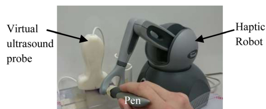
Fig. 1 Prototype haptic robotic CVC trainer with virtual ultrasound probe, haptic needle, and scanning surface
