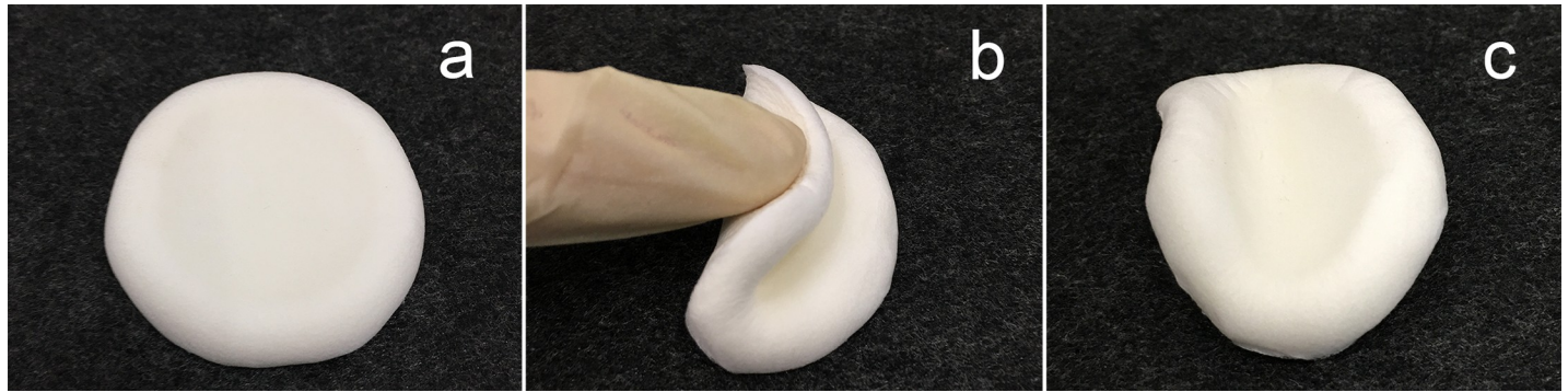
Fig 2. Morphology of the composite sponge. (a) flattened sponge, (b) folded sponge, (c) recovered sponge.
