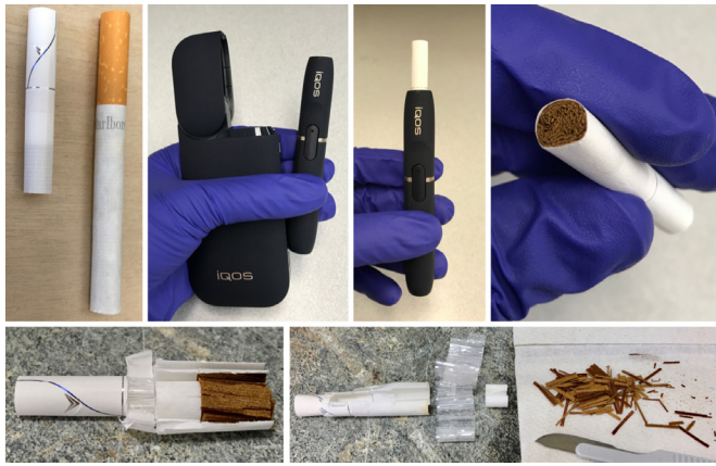
Figure 1 IQOS. IQOS is composed of three main parts: HeatStick, holder and pocket charger. HeatSticks are inserted in the holder, which contains an electronic heating blade to heat tobacco and release aerosol. HeatSticks contain strips of processed and reformed tobacco. Photos by MLS and PN.
