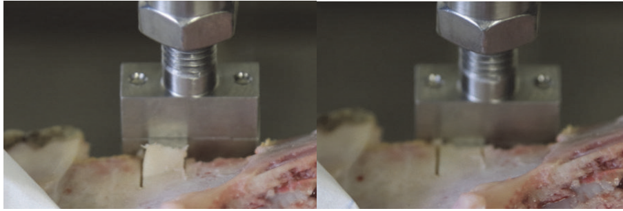
FIGURE 4: Biomechanical testing with a servo-electric material testing machine demonstrating fracture of the split lamella on the right side.
