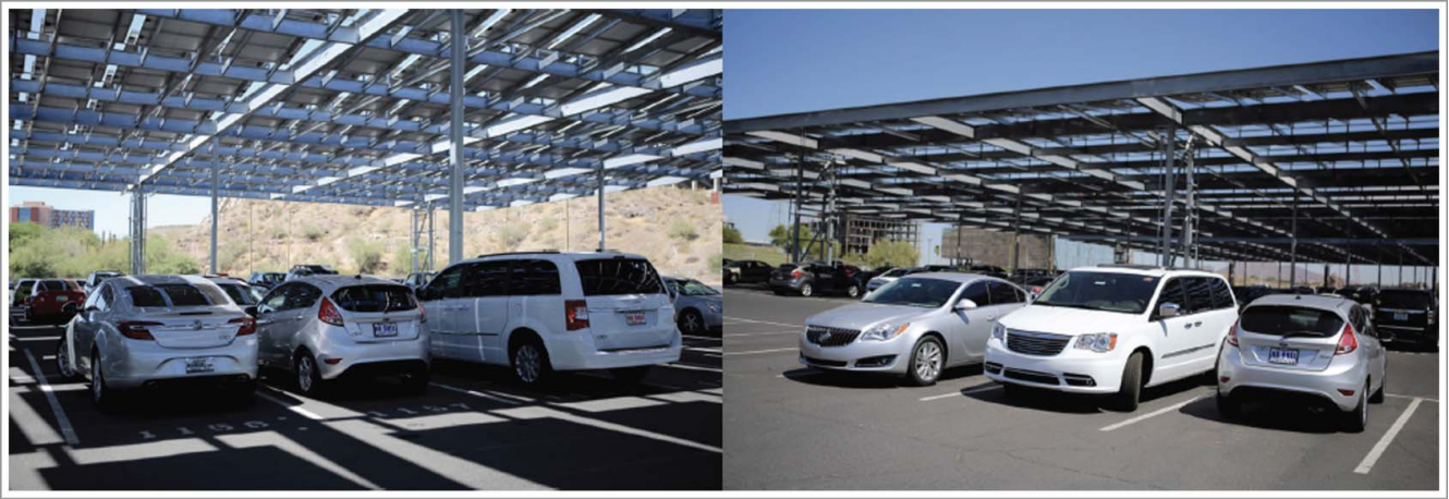
Figure 1. Exposure of vehicles (Midsize Sedan, Minivan, Economy Car) shaded by a solar structure (left) and of those in the direct sun (right).
