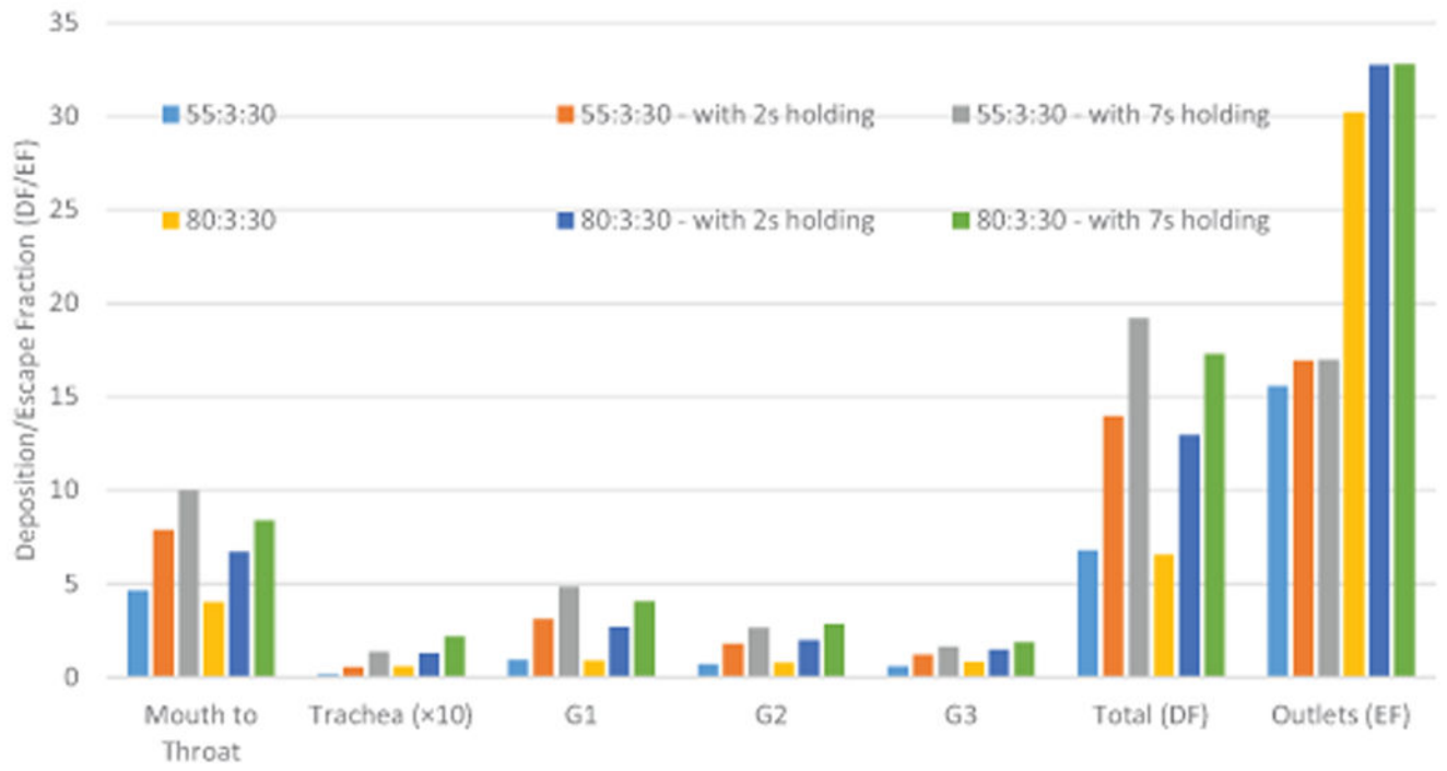
Figure 7: Comparisons of EC particle deposition fractions in the idealized human upper airway model.
