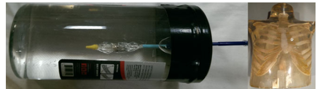
FIG. 8. Experimental setup for C-arm CT acquisitions. Left: Sapien XT 26 mm valve is mounted on an inflatable balloon catheter within a water-filled cylindrical container. The catheter is guided through a sealed hole in the lid of the container. Right: Chest phantom used for anatomical background. [Color figure can be viewed at wileyonlinelibrary.com]
