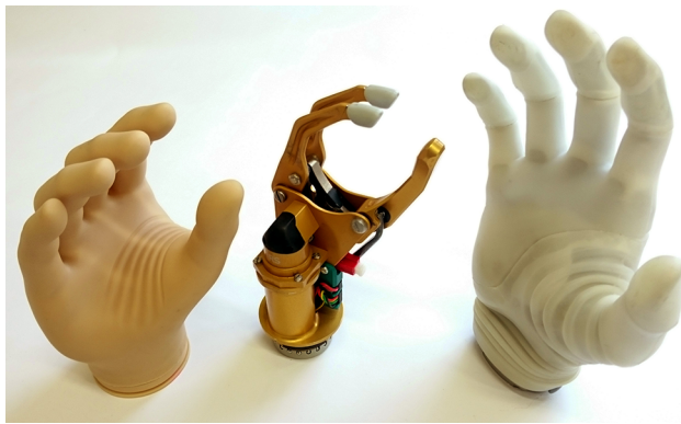
Figure 1 Examples of Ottobock prosthetic hands and cosmetics (from left to right): small System Inner Hand, small MyoHand VariPlus Speed, and medium Michelangelo hand.
