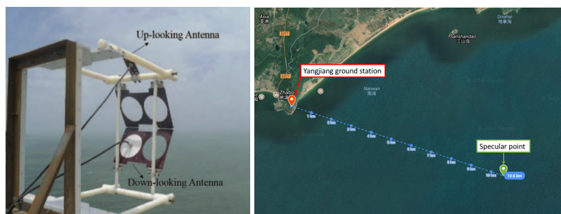
Figure 2. The ground receiving station at Yangjiang site to collect the reflected signal from the BeiDou G4 satellite. Up and down-looking antenna (left) and the distance between receiving station and specular point (right).
