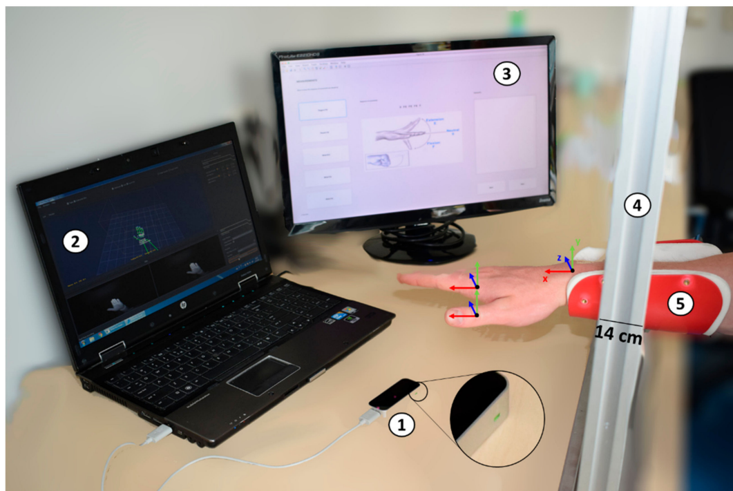
Figure 1. Experimental setup. (1) The controller of the Leap sensor. The green light indicates that the controller is on. (2) Brekel Pro Hands application in real-time, on the host computer. (3) The Guide User Interface shows which movement the participant should do. (4) The platform with (5) arm support at a distance of 14 cm from the table's surface, where the participant should place his forearm.
