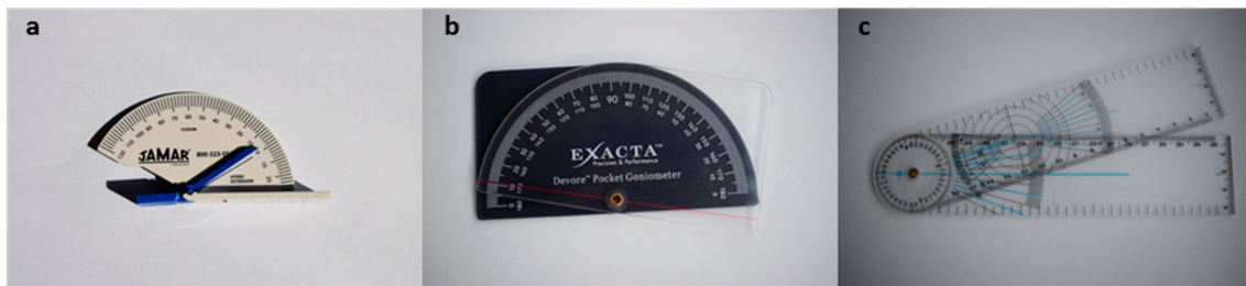
Figure 3. Goniometers used in this study: (a) Rolyan finger goniometer with loose-fitting hinge; (b) Devore pocket goniometer; and (c) universal goniometer with full-circle body.
