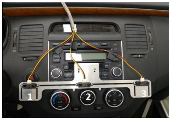
Figure 4. Positions of infrared sensors on the center console.
