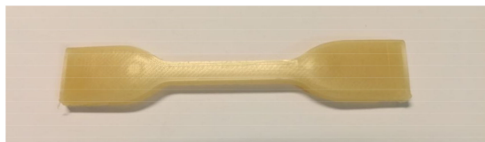
Figure 8. 3D printed dogbone for tensile tests (PHB/PLA/A-4).
