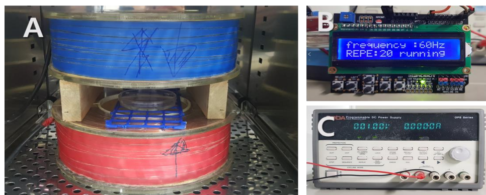
Figure 4. Photograph of the electromagnetic field (EMF) device in incubator. Pulsed EMF was generated using a pair of Helmholtz coils. (A) Helmholtz coil; (B) function generator; (C) power supply.
