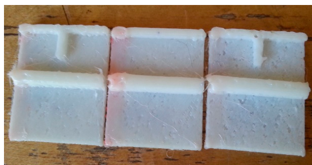
Figure 2. Test samples produced with fused deposition modeling (FDM) using travel speeds of the extruder (left to right) of 15, 20, and 30 mm/s.
