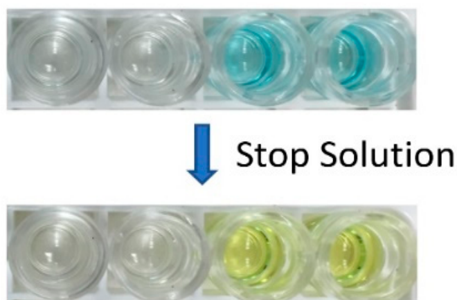
Figure 6. Colorimetric bioassay results after the stop solution is added. The wells with the blue solution are the positive controls and the colorless wells represent the negative controls.
