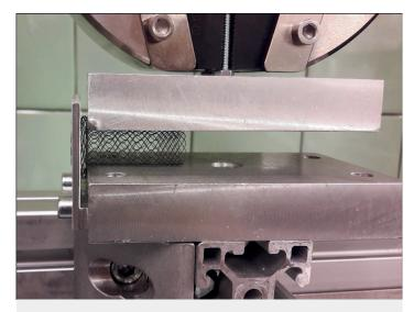
*Figure 1.* Testing of global compression. The stents were compressed between plaques up to 50% at a compression rate of 2 in/min.
