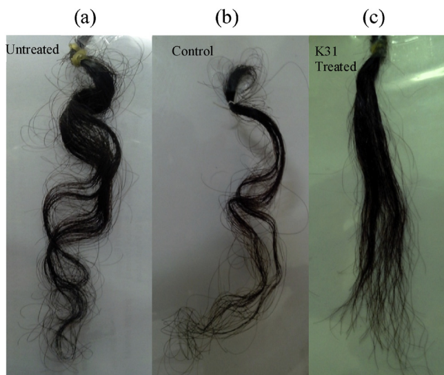
Fig. 4. Application of keratin K31 in straightening curly hair. (a) Untreated curly hair; (b) curly hair after alkali treatment and washing; (c) alkali treated and washed hair after keratin K31 treatment.
