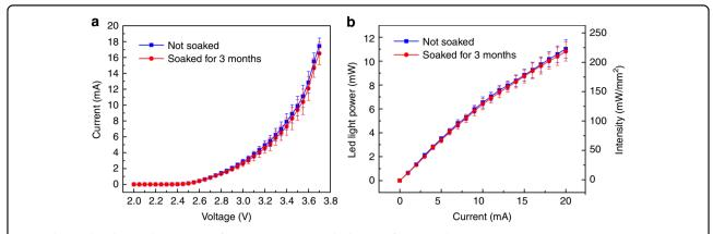
Fig. 5 Electrical and optical properties of micro-LED arrays soaked in PBS for 3 months. a /-V mean value curves with standard deviations measured from 32 micro-LEDs on two samples. b Mean value and standard deviation of light output power and intensity of the same two samples
