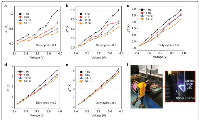
Fig. 6 Thermal property of the integrated single micro-LED on the array. Duty cycle from 10–90% (a–e), frequency from 1 to 50 Hz, and voltage from 2.5 to 3.9 V; dashed line at  $\Delta T = 2$  K indicating the maximum acceptable temperature increase to avoid thermal damage of brain tissue. f Measurement setup with an IR thermal imager with the enlarged view of the micro-LED array facing the macro IR lens
