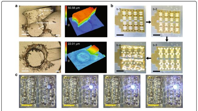
Fig. 3 Silver paste-aided wire-bonding on the flexible substrate and its effect. a Two states of second bonding joint on polyimide substrate: disconnected (above) and connected (below). **b** Flow photos of the micro-LEDs' setup and package showing the silver paste-aided wire-bonding. **c** Actual working effect of a single micro-LED under different voltages (2.6–3.8 V). All scale bars in **b** and **c** are 1 mm
