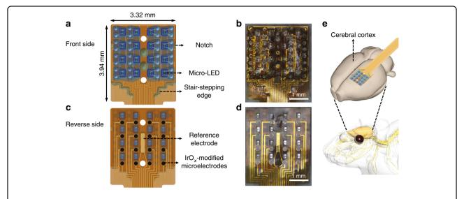
**Fig. 1 Design schematic of the opto-electric neural interface. a** Schematic diagram and **b** photograph of the front side of the assembled device with 16 micro-LEDs on the top, **c** schematic diagram and **d** photograph of the reverse side of the assembled device with 16  $IrO_x$ -modified microelectrodes on the top, and **e** the sketch of the device attached on the cerebral cortex of a rat
