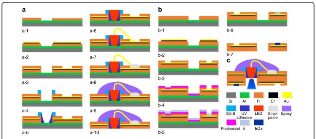
Fig. 2 Fabrication processes. a The micro-LED array and b the micro-ECoG electrode array based on polyimide substrate. c Assembled device with the micro-LED array stacked on the micro-ECoG electrode array
