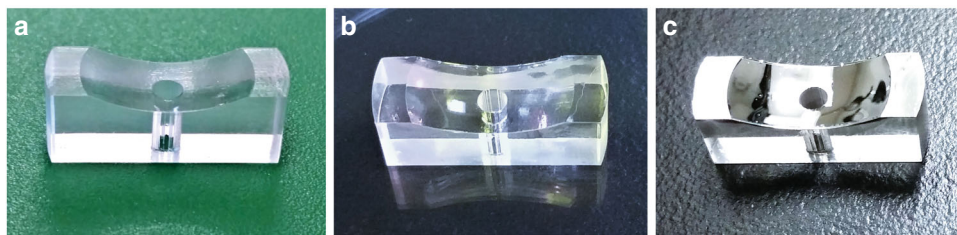
Fig. 2 3D printed parabolic mirrors at different stages of the fabrication process. As printed (a), after smoothing (b), and the completed mirror after smoothing and Al deposition (c)
