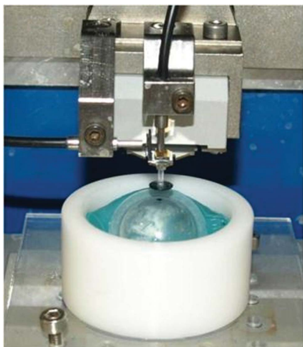
FIG. 1. Position of the CL for peripheral region CoF measurement. CL, contact lens; CoF, coefficient of friction.
