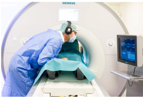
Fig. 1 Current situation: A radiologist performs an MRI-guided needle puncture while using a separate display outside the MRI bore
