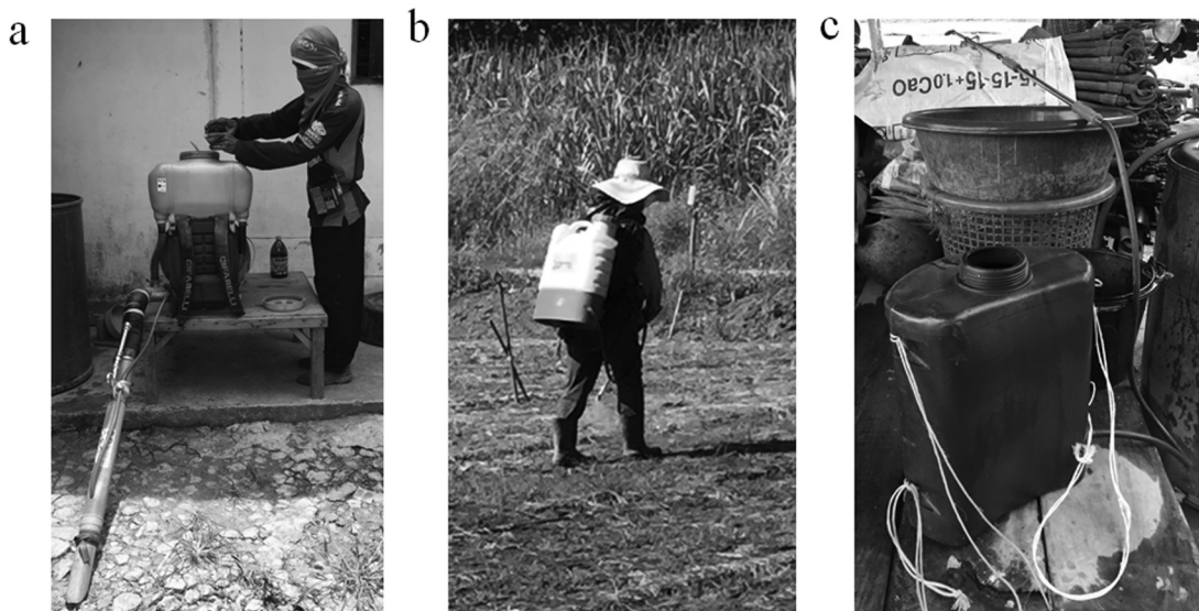
Figure 1. Type of spraying equipment: (a) 2 stroke gasoline motor and fan, (b) a battery operated pump and (c) a manual hand pump.
