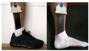
**Figure 3** *Experimental shoes (left), barefoot (right), and the set-up of the plantar pressure system.*
