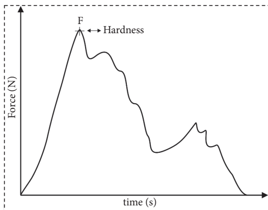
FIGURE 2: Typical curve of force (N) versus time (s) showing the maximum compression force used for describing the snack texture.
