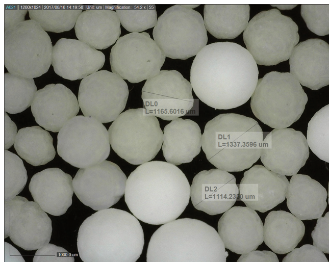
Figure 1: Measurement of pellet size. Dummy particles seen as perfectly smooth round pellets with a different color compared with the surrounding drug-coated pellets
