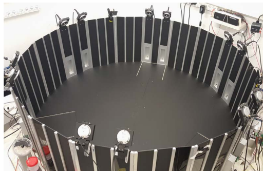
Fig. 1. The echoic environment. An image of the echoic arena. 12 speakers are spread in pairs around the arena wall.
