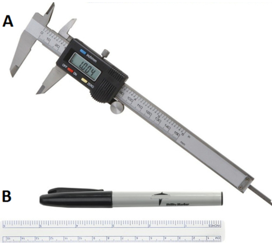
Figure 2. Measuring instruments. A) Digital caliper. B) Sterile utility skin marker and ruler. Please click here to view a larger version of this figure.
