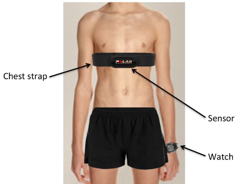
Figure 1: Diagram of heart rate technology, depicting optimal placement of chest strap, sensor and watch. Please click here to view a larger version of this figure.
