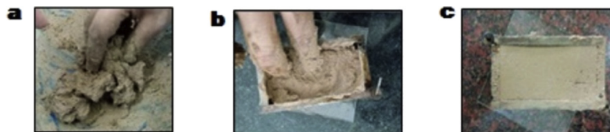
Fig. 2. (a) mixing of materials (b) filling into the mould (c) levelling of surface.
