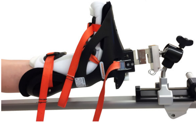
Figure 1. Image of the custom attachment that was created to allow integration of an S-type load cell into the traction system. The patient was positioned on the surgical table and traction system. After anesthesia induction, a fluoroscopic image was obtained to define the pretraction joint position. Traction was then applied to the surgical limb, and a second fluoroscopic image was acquired in the same plane to confirm that sufficient distraction had been achieved to allow completion of all components of hip arthroscopic surgery in the central compartment. Traction force was continuously measured through this process.
