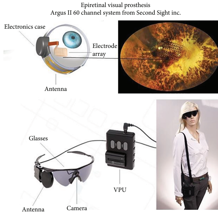
FIGURE 2: Epiretinal visual prosthesis consists of a highly flexible electrode array tacked onto the inner surface of the retina, which is connected to a multichannel stimulator that is strapped to the eyeball and receives power and command signals from an external video camera and video processing unit (VPU) via an externally generated radio-frequency magnetic field. Photos used with permission of the manufacturer, Second Sight Inc., Sylmar, CA 91342.
