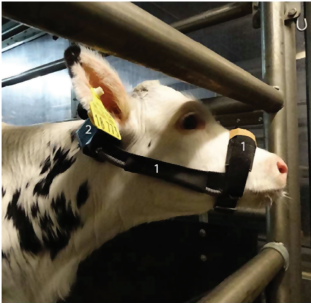
Figure 1. The RumiWatch System (RWS; ITIN + HOCH GmbH Feeding Technology, Liestal, Switzerland) composed of a halter with a noseband sensor comprising of an oil-filled silicon tube reaching from the left to the right side of the nose and the right cheek to end up in the pressure sensor (1). Behind the right ear, a box comprising the accelerometer, the battery, the data logger, and a SD card was fixed to the halter (2). Data recorded by the device are converted to an Excel file using the corresponding evaluation software (version 0.7.3.2).
