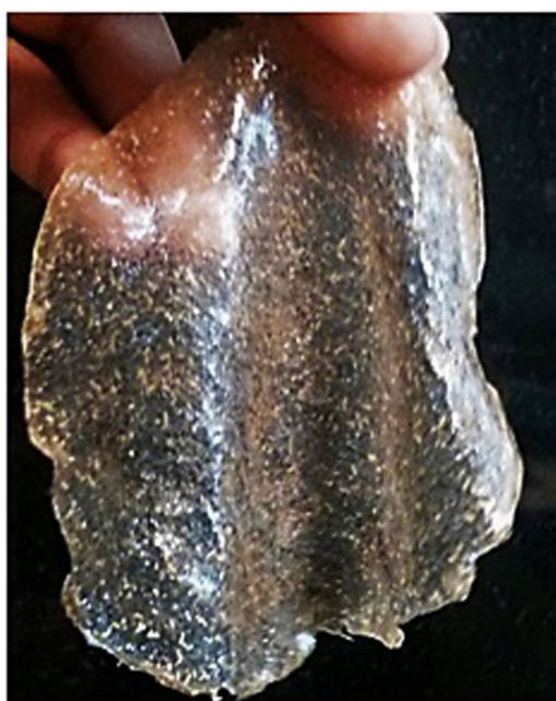
Figure 3. Picture of a lauroyl grafted alginate-Psyllium husk gel non-adhesive composite film.
