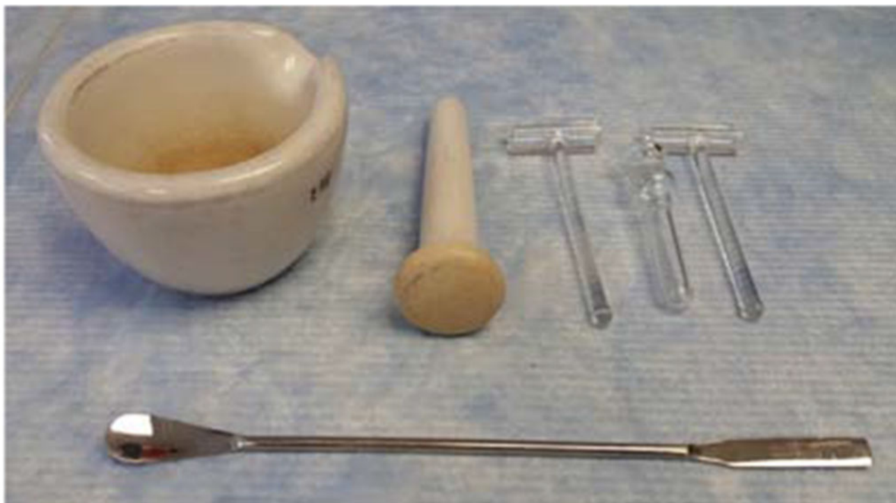
FIG. 1. Equipment used for pulverizing bone fragments. Top left is a mortar and pestle; top right is the glass homogenizer; bottom is a spatula.
