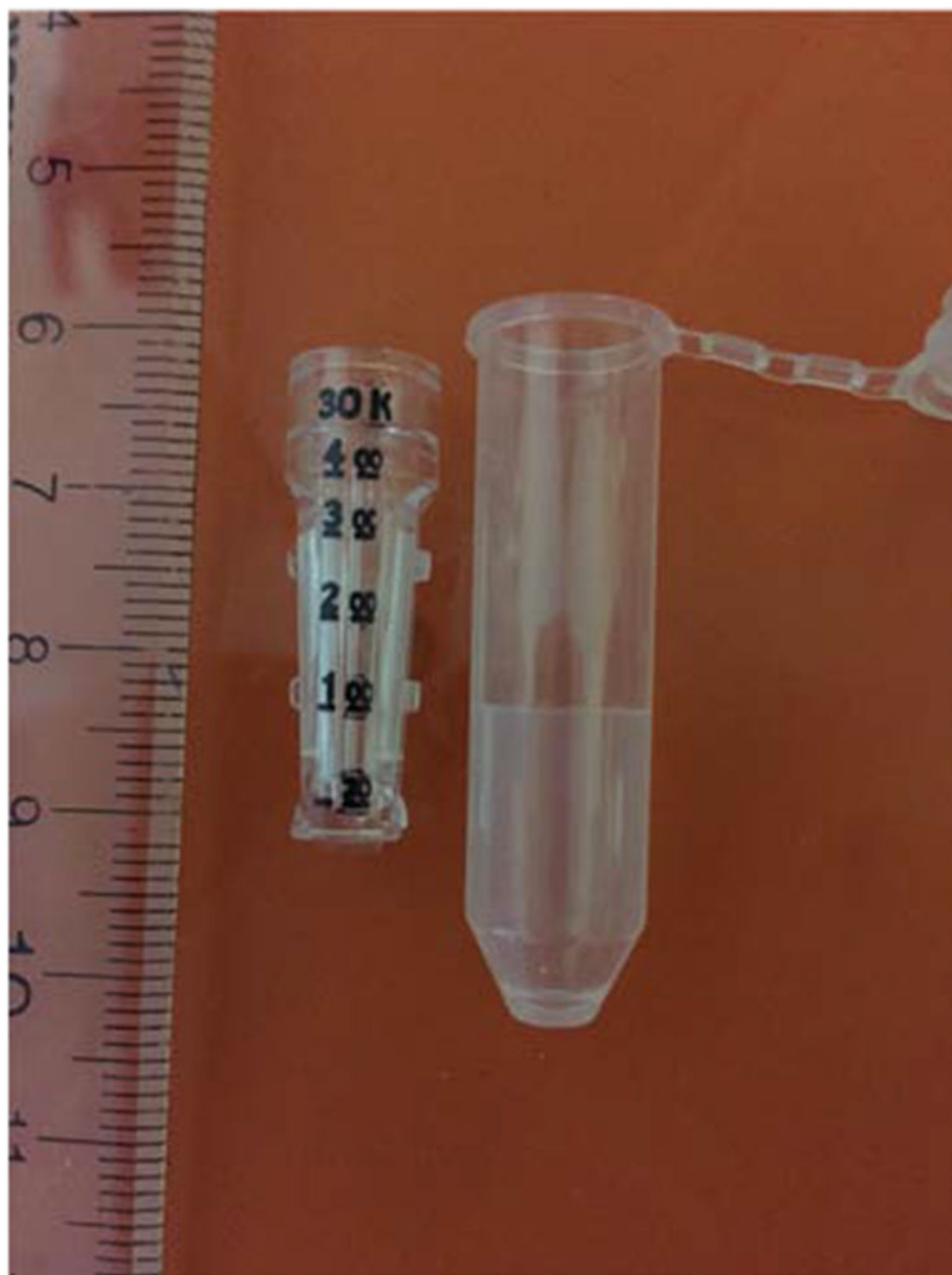
FIG. 3. Amicon centrifugal filter in tube. 30K MW is preferable when working with SLRPs.
