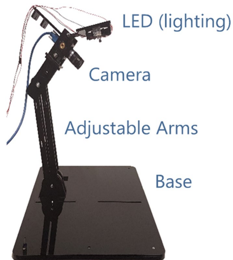
Figure 2. The camera rig used to record the videos from the JV pulsation of the subjects. The two movable arms helps to adjust the camera position relative to the neck. A blue LED was used to illuminate the location of the recordings.
