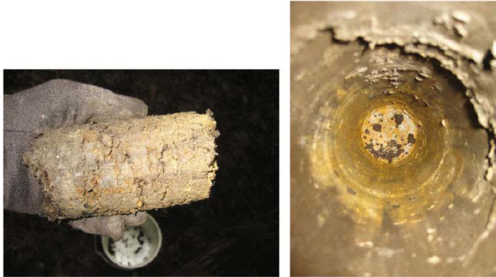
Fig. 3. Cores sampled from sites in the Erie Drift Plain (EDP) appeared to have substantial clay fraction of the soil, which may provide sorption sites for available phosphorus, although this was not ascertained in the study. The left panel is an example of the cores extracted from EDP, whereas the right panel is a picture looking downward into the core hole.
