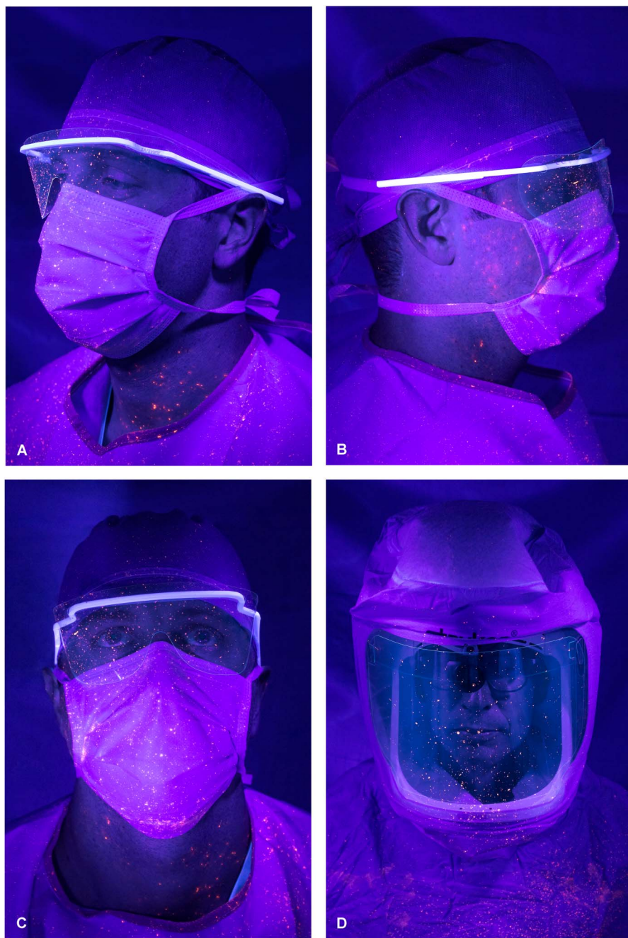
Fig. 4A-D Particulate matter exposure encountered by surgical participants while wearing each gowning system shown here, including side views (A-B) and front view (C) of conventional gowning systems, and front view of the positive-pressure exhaust suit providing complete surgical participant protection (D).
