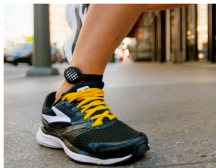
Figure 5. This figure shows the Moov Now device that contains nine-axis motion sensing. Image source: [29].
