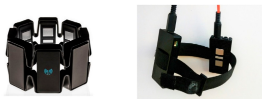
Figure 3. This figure shows the Myo band on the left and two EMG channel sensors on the right. Image source: [21,22].
