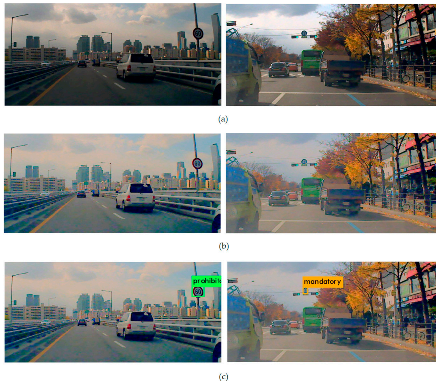
Figure 3. (a) Original dark images; (b) improved luminance by tone mapping; and (c) detection of traffic signs.
