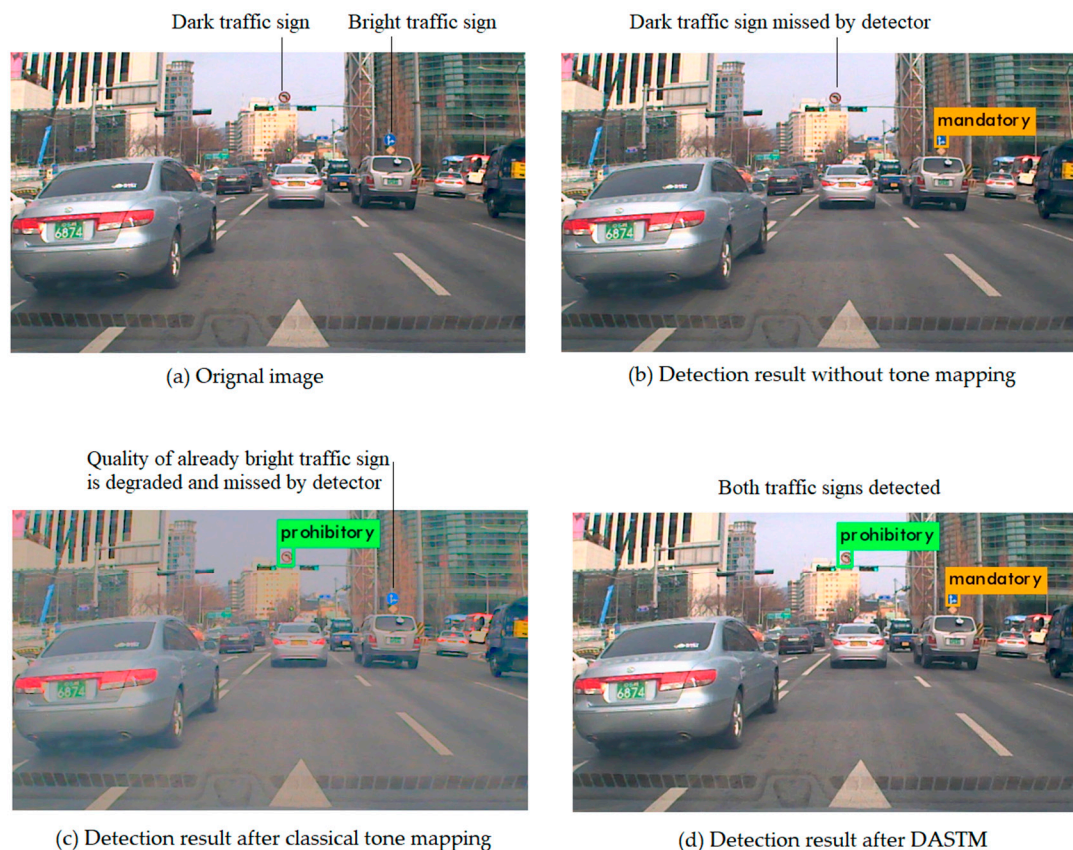
Figure 2. Typical results of detection: (a) original image; (b) detection without tone mapping, in which a dark traffic sign is missed; (c) detection after classical tone mapping, in which a bright traffic sign is missed; and (d) detection after DASTM, in which both traffic signs are successfully detected.
