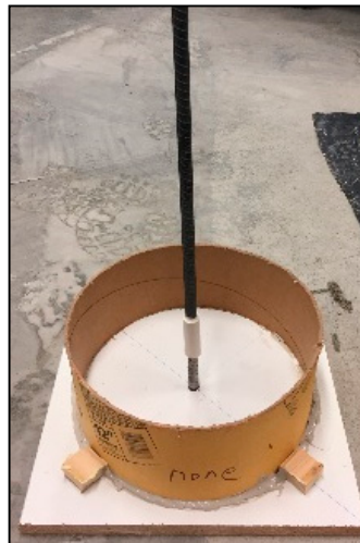
Figure 2. Pull-out test specimen.
