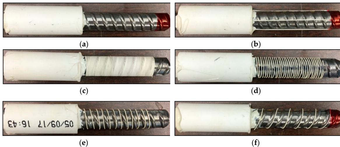
Figure 3. Photograph of steel bars in concrete cylinders for pull-out test: (a) Ref; (b) L4; (c) S0; (d) S2; (e) S5; (f) S10.
